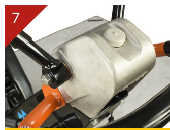
Large Volume Oil Tank
