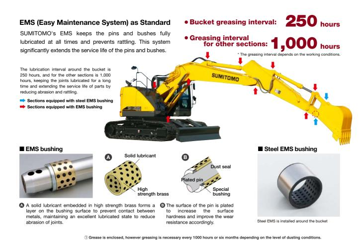
② Greasing is also necessary after any components have been submerged underwater for prolonged periods.
