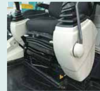
Seat suspension absorbs vibration
