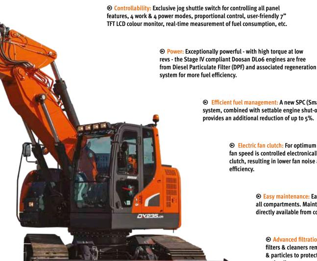
**⊙** Efficient fuel management: A new SPC (Smart Power Control) system, combined with settable engine shut-off & auto-idle,
