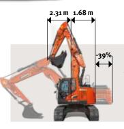
Reduced tail swing radius: To facilitate use in the city and in tight locations, the tail swing radius is 39% shorter compared to the conventional DX235LC-5. The smallest swing diameter is only 3.99 m.
