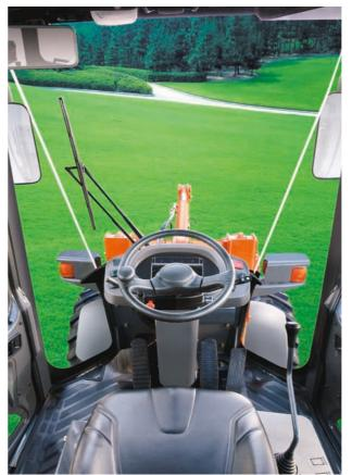
Uses a large sliding sash for the door and a pillar-less design gives an unobstrusted view of the front. The cab enables panoramic views via the addition of a lower window, which was absent in existing models, the removal of the rear corner pillar, and the use of a new and improved defroster nozzle, etc., providing a wide field of vision.
