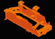
To reinforce the front and rear frames, a box-section structure has been introduced. This improves durability, which results in greater reliability.
