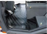
The area around the door has been redesigned to produce a flat, even floor inside the cab. This allows for easy of cleaning.
