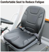
A comfortable seat to relieve operator fatigue has been adopted. Absorbs unpleasant vibrations, reduces psychological and physical burdens, and reduces fatigue due to long time operations.
