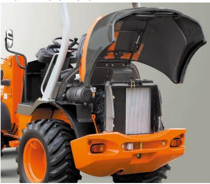
Daily maintenance is even easier with the incorporation of a large full-open cover and lowest counterweight. The cover opens at a touch, and is supported by tow gas dampers. The engine room, which can be fully open, enables maintenance such as inspections, replacements and filling to be carried out with ease.
