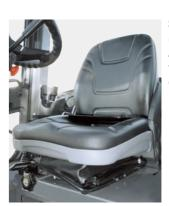
**Suspension Seat** (Optional) A suspension seat is available to lessen vibrations and shock during operation.
