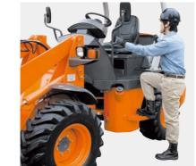
There are handrails and large steps mounted on both the left and right of the cabin for easy access.
