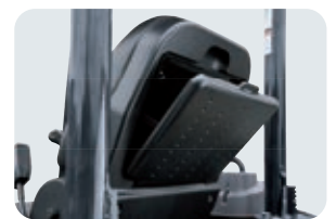
Comes equipped with a operator's manual case at the back of the seat.
