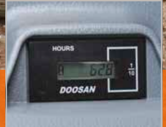
Hour meter (from ground level)
