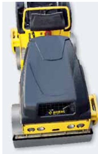
100% “clear-sided” models with drums free on one side giving an offset of 60 mm.
